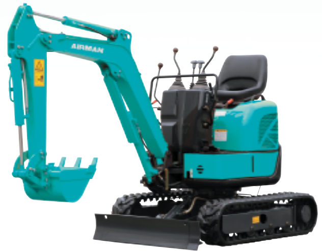
AX17u-4 Supports 3-pillar canopy ROPS/OPG (TOP guard)
